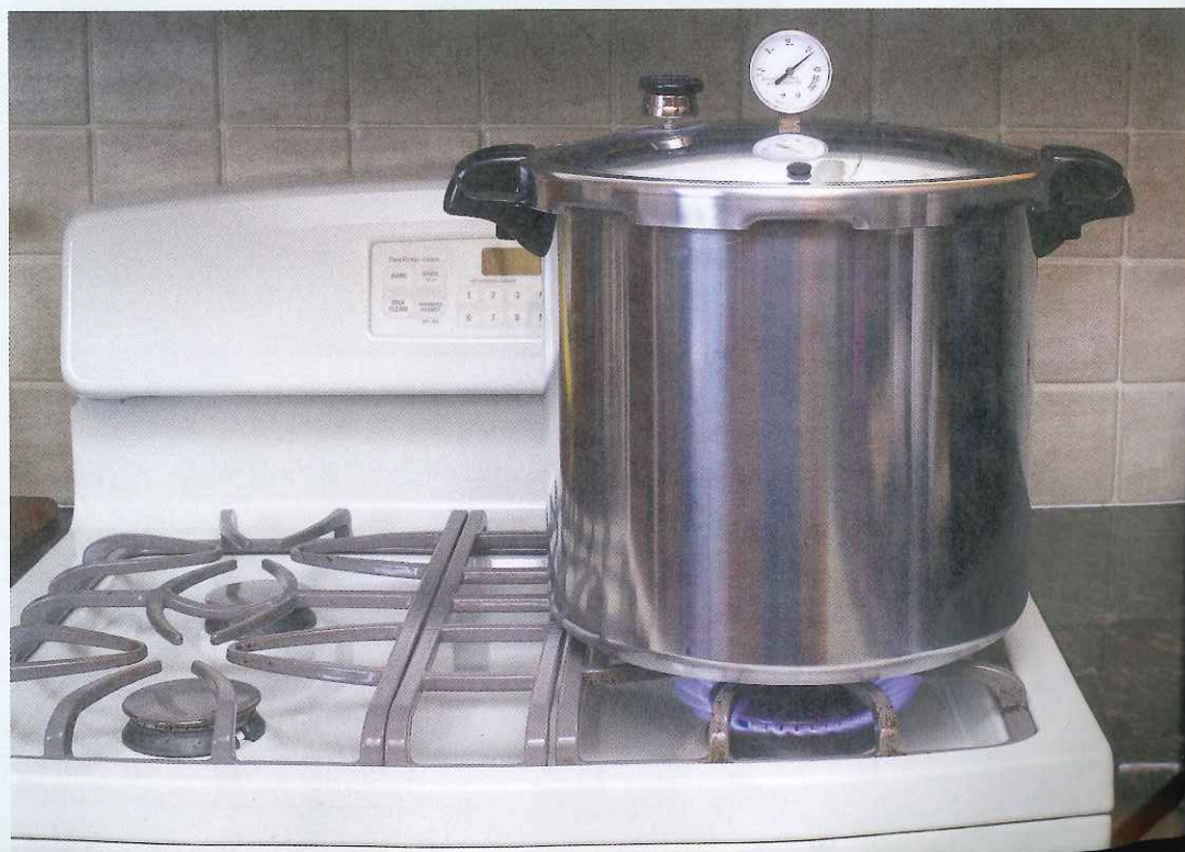
Figure 14.12 Pressure Cooker A pressure cooker is a gas-tight container in which pressurized steam is used to cook food. With the lid locked, the volume of steam and the number of water molecules are constant. So any increase in temperature causes an increase in pressure.
