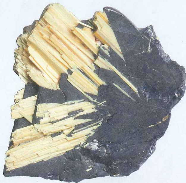
Figure 7.10 Rutile Titanium dioxide, or rutile, forms tetragonal crystals. In \text{TiO}_2 , each \text{Ti}^{4+} ion has a coordination number of 6, while each \text{O}^{2-} ion has a coordination number of 3.
