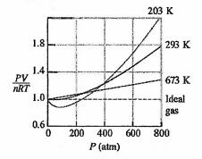
This graph is just for nitrogen gas. Note that although nonideal behavior is evident at each temperature, the deviations are smaller at the higher Ts.
