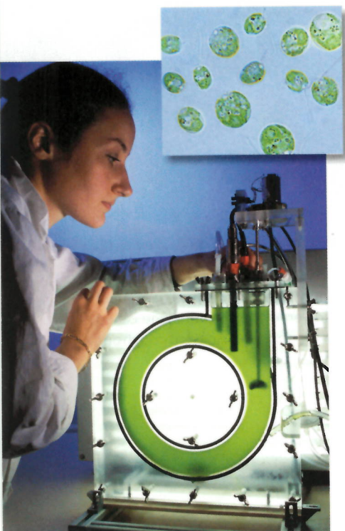
FIGURE 1.19 Biotechnology is being used in the search for alternative energy sources, as shown in this bioreactor that uses algae (inset) to produce hydrogen gas. (LM; magnification 400×)
