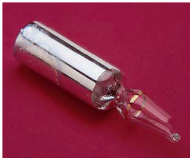
A vial containing potassium metal. The sealed vial contains an inert gas to protect the potassium from reacting with oxygen.
