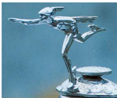
Chromium is often used to plate bumpers and hood ornaments, such as this statue of Mercury found on a 1929 Buick.
