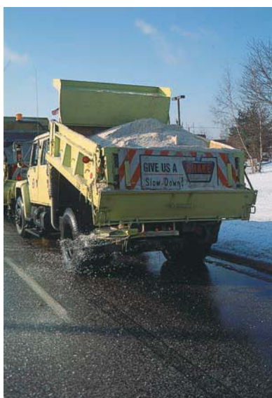
Spreading salt on a highway.
