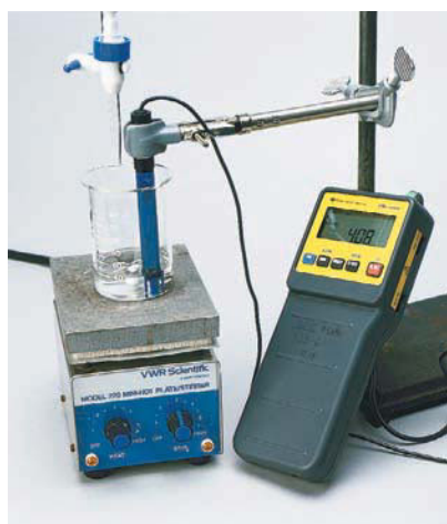
A setup used to do the pH titration of an acid or a base.
