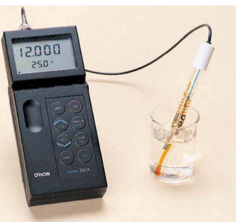
(top) Pure water at pH 7.000. (bottom) When 0.01 mol NaOH is added to 1.0 L of pure water, the pH jumps to 12.000.
