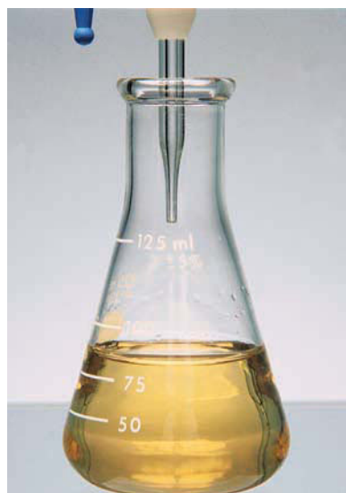
Methyl orange indicator is yellow in basic solution and red in acidic solution.
