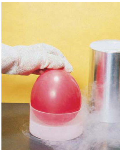
(a) A balloon filled with air at room temperature. (b) The balloon is dipped into liquid nitrogen at 77 K. (c) The balloon collapses as the molecules inside slow down due to the decreased temperature. Slower molecules produce a lower pressure.
