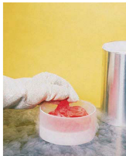
(a) A balloon filled with air at room temperature. (b) The balloon is dipped into liquid nitrogen at 77 K. (c) The balloon collapses as the molecules inside slow down due to the decreased temperature. Slower molecules produce a lower pressure.
