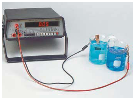
A concentration cell with 1.0 M Cu 2+ on the right and 0.010 M Cu 2+ on the left.
