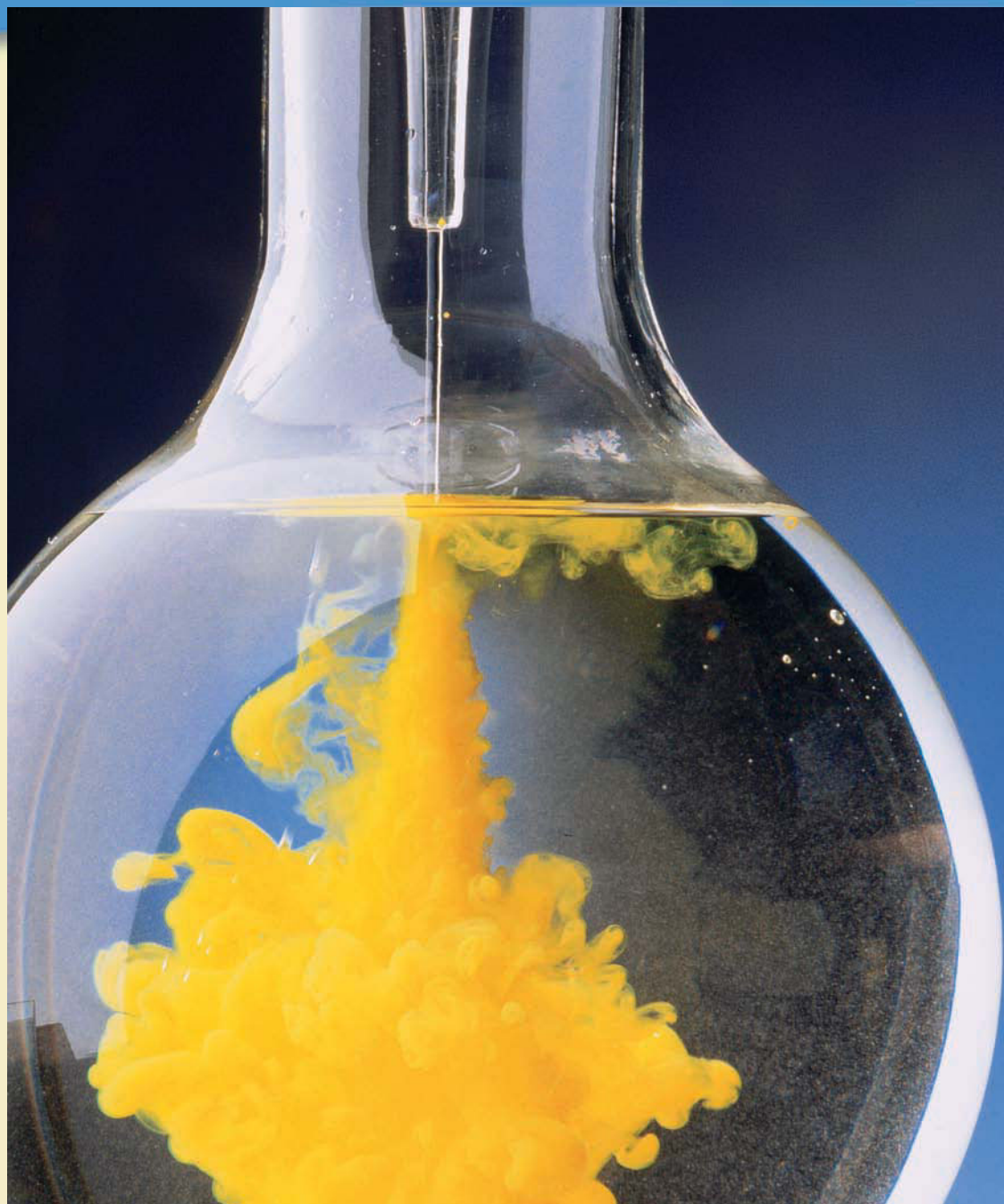
Yellow lead(II) iodide is produced when lead(II) nitrate is mixed with potassium iodide.
